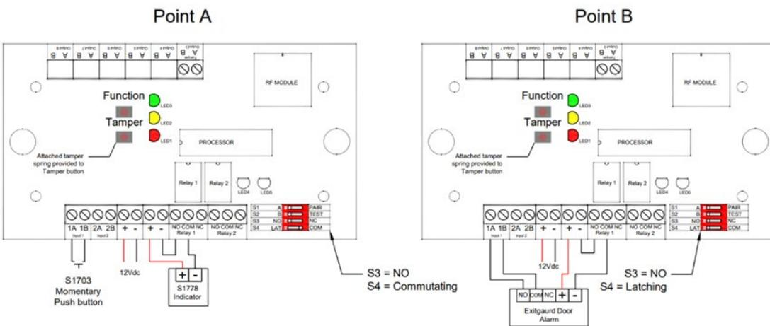
In this scenario a momentary push button at point A would wirelessly arm the Exitguard door alarm at point B.
