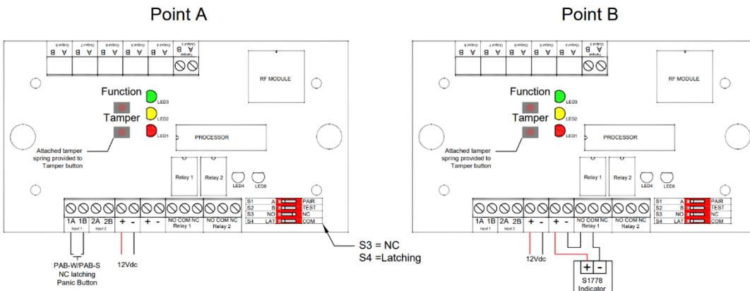
In this scenario a latching panic button at point A would wirelessly trigger and indicator at point B.
