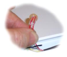
Visually check there is a good connection with both wires
