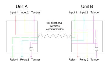
The Wireless Relay system has many applications where short range transmission of simple switches is required, for example, PA buttons, door contacts, remote sounders, lighting, door locking etc. The units are supplied in double gang plastic plates.
