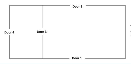
Three door two door interlock example with door 3 common to both interlocks.
