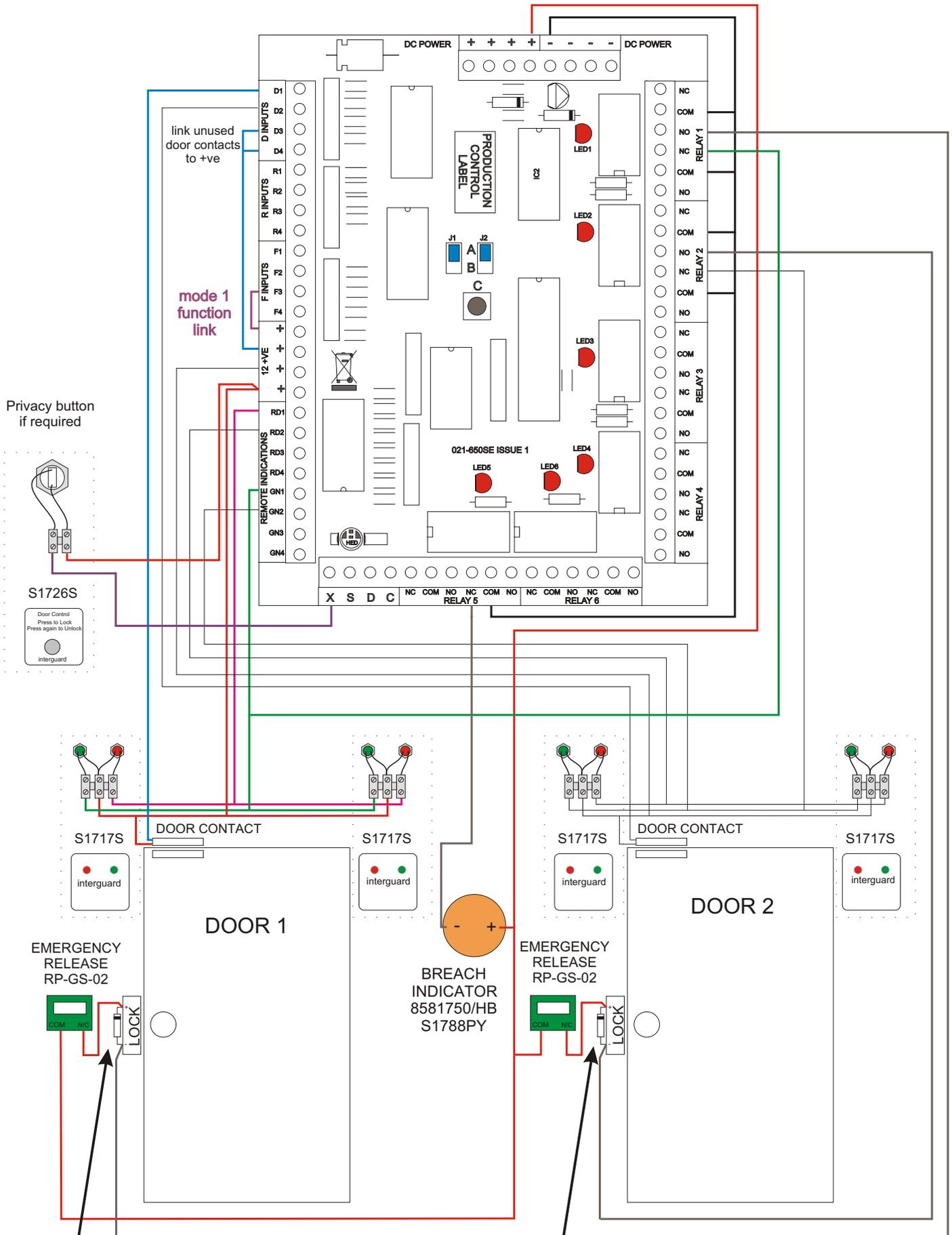
NOTE. Fit back EMF protection diode to magnetic lock.
