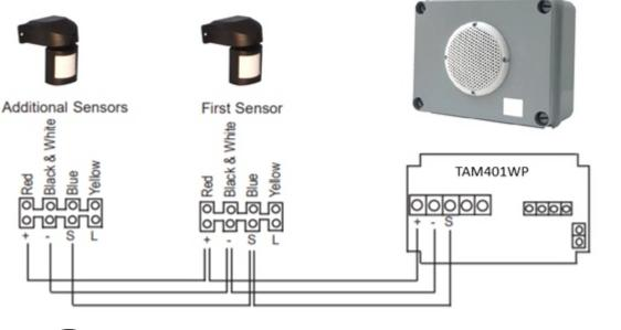
Works in conjunction with TAM401WP. Eight different voice messages can be played by activating one of the Eight inputs. Multiple sensors could be installed to enable different voice messages to be played on the Chatterbox TAM401WP
