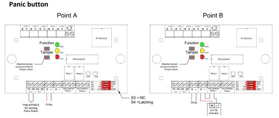
In this scenario a latching panic button at point A would wirelessly trigger and indicator at point B.
