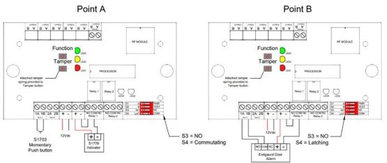
In this scenario a momentary push button at point A would wirelessly arm the Exitgaurd door alarm at point B.
